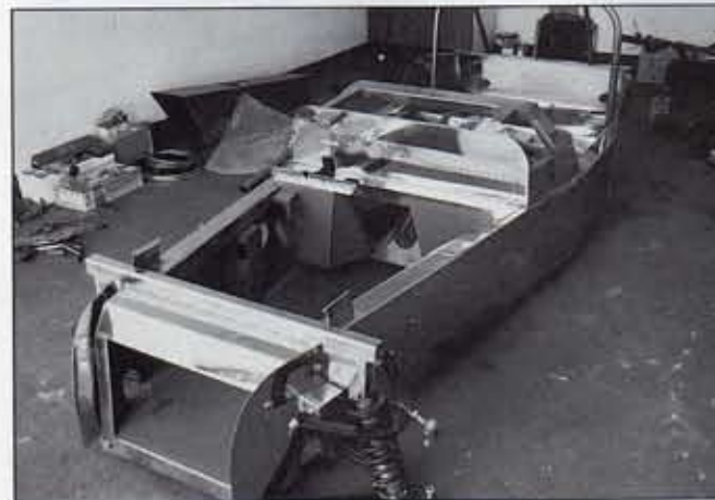
Above: Stainless monocoque was to prove immensely rigid on the road. We opted for the Robin Hood front suspension package. Below: Engine and gearbox being lifted in. Very quickly up to a rolling chassis.
