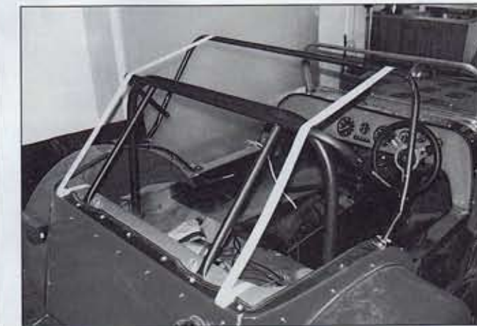
Above: Trimming the dash with foam padding and then vinyl. Edges were stapled into place. Below: Sorting out the hood support rail positions. Cord holds everything in place and can be easily adjusted.
