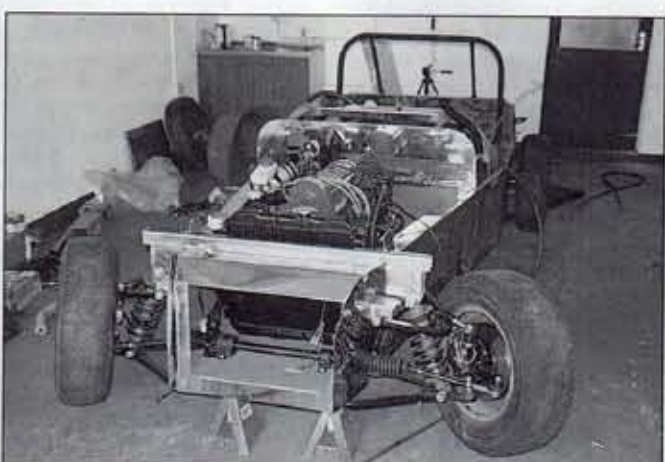
Above: Carefully fixing brake line and wiring loom to the floor and away from the propshaft. Central tunnel encloses everything. Below: The rolling chassis was very quickly completed.
