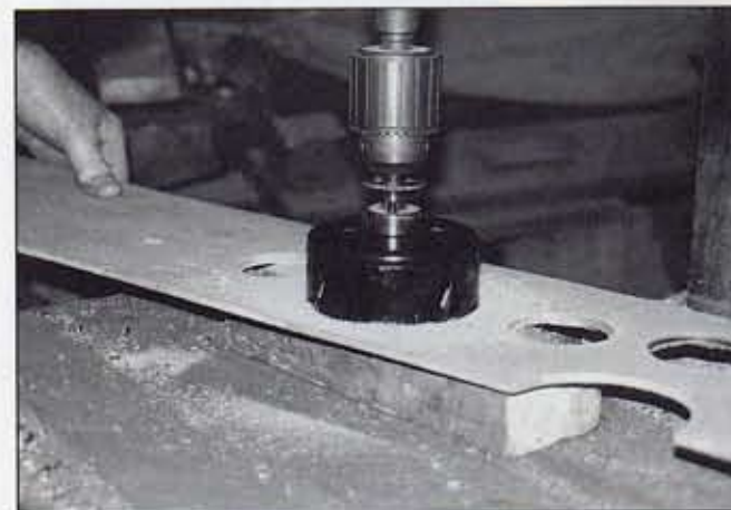
Above: Cutting out the holes in the dashboard using a neat hole cutting saw. A very useful and quite cheap piece of kit. Below: Modified Cortina instrument pod is neatly disguised behind the dash.
