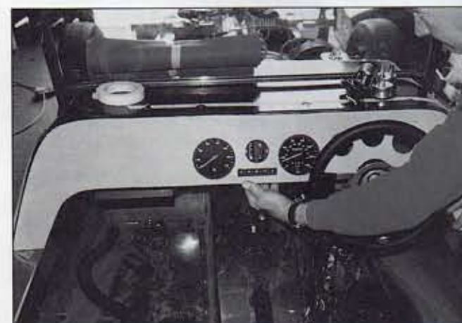
Above: Cutting out the holes in the dashboard using a neat hole cutting saw. A very useful and quite cheap piece of kit. Below: Modified Cortina instrument pod is neatly disguised behind the dash.
