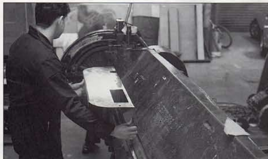
Below: The old and new. Massive sheet folder makes light work of stainless panels. CAD controls plasma cutter and maximises use of sheets.
